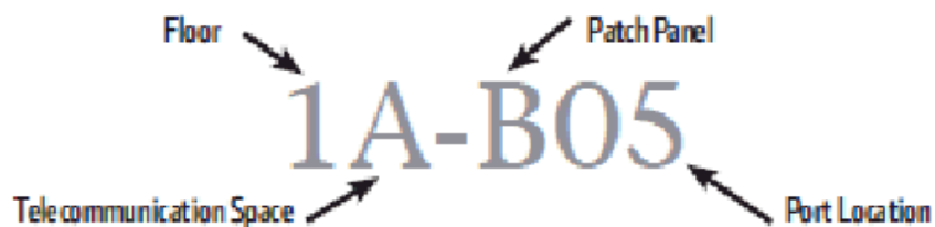
Figure 1: A workstation outlet labeled per TIA-606-A horizontal link identifier
